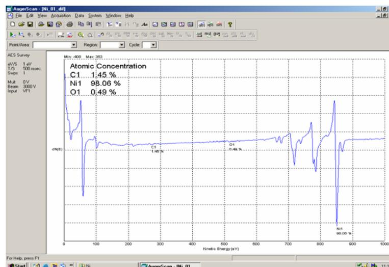
Figure 7. The results of measurements of C and O concentrations in Ni coatings of 2.5  $\mu$ m using Auger electron spectroscopy (AES) techniques. Values of 1.45%C, 0.49%O have been obtained.
