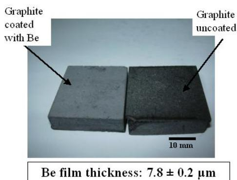
Figure 9. Photograph of a Be coated and an uncoated graphite sample.
